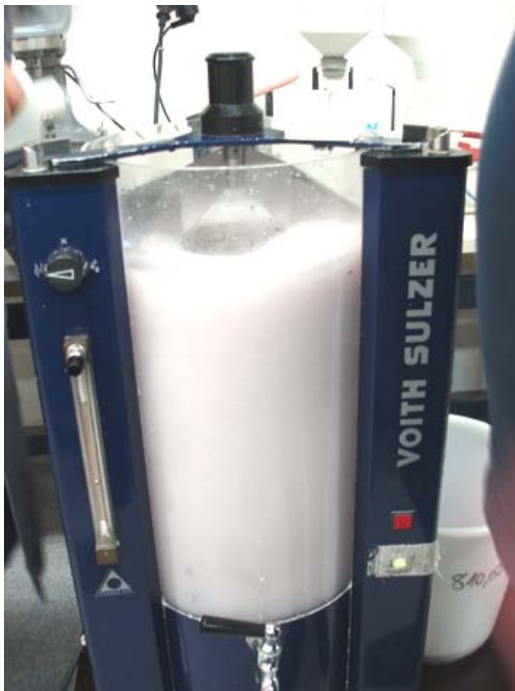
Deinking by flotation
