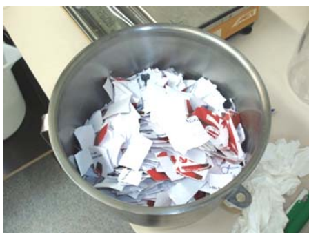
Printed product sample is pulped with standard deinking recipe in the Hobart pulper
