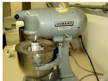
Printed product sample is pulped with standard deinking recipe in the Hobart pulper
