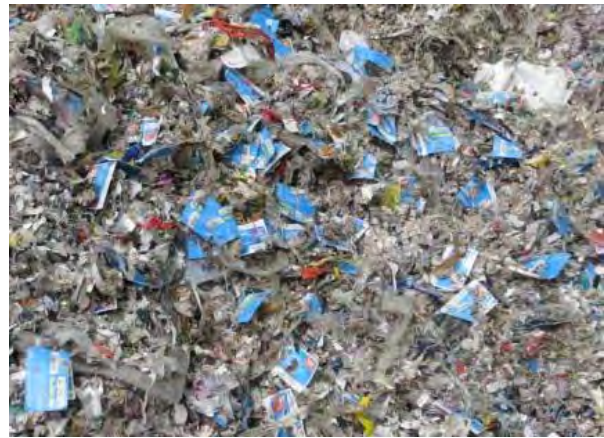
Plastic cards in the coarse reject of a deinking plant
