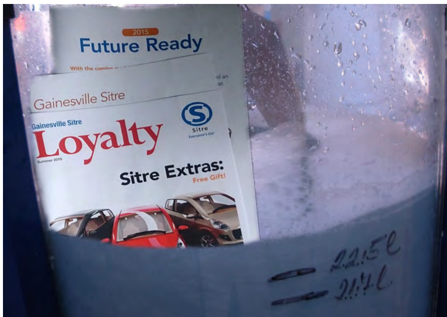
Not ready for the future: Prints from the Impika Evolution inkjet printer are not suitable for deinking, the dissolved pulp stays dark even after seven minutes of flotation in the lab.
