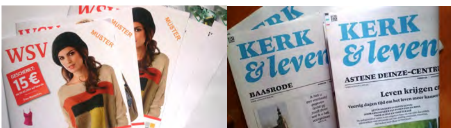
A barely deinkable sample (Canon Océ Colorstream 3000Z, left) and one not suitable for deinking (Colorstream 3900).
