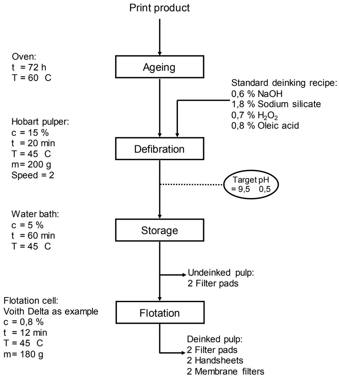
**Figure 3: Procedure for testing deinkability with standard deinking recipe**
